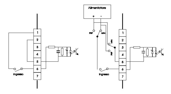
The inputs can be type NPN or type PNP, according to the polarization of the connecting terminal number 5.
