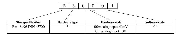
Warning: On the order, you must specify the power voltage of the instrument which can be 24-110-220 VAC
